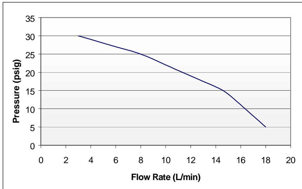
Figure 4 – Zero-Air Generator Performance Curve
