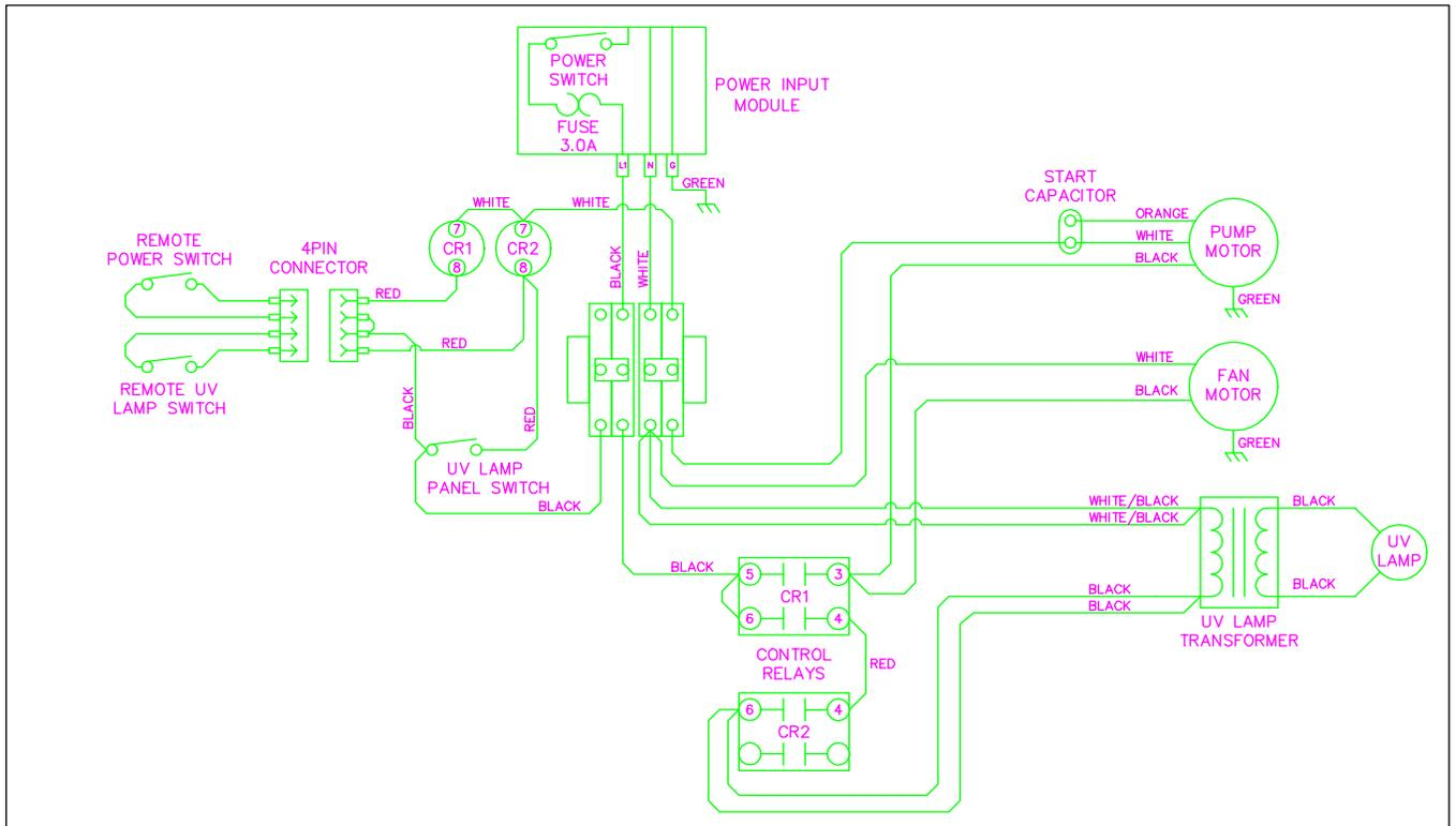
Figure 5 – ZAG Wiring Schematic
