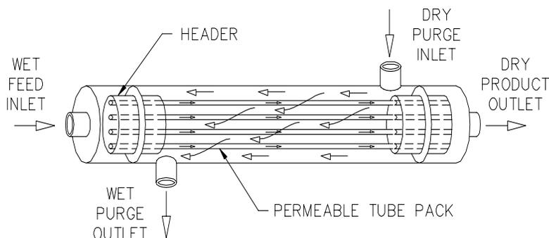
Figure 2 – Perma Pure Nafion Membrane Dryer Schematic
