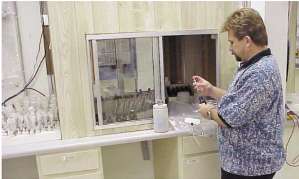
*Ventilation Hood for Calibration Procedures*
