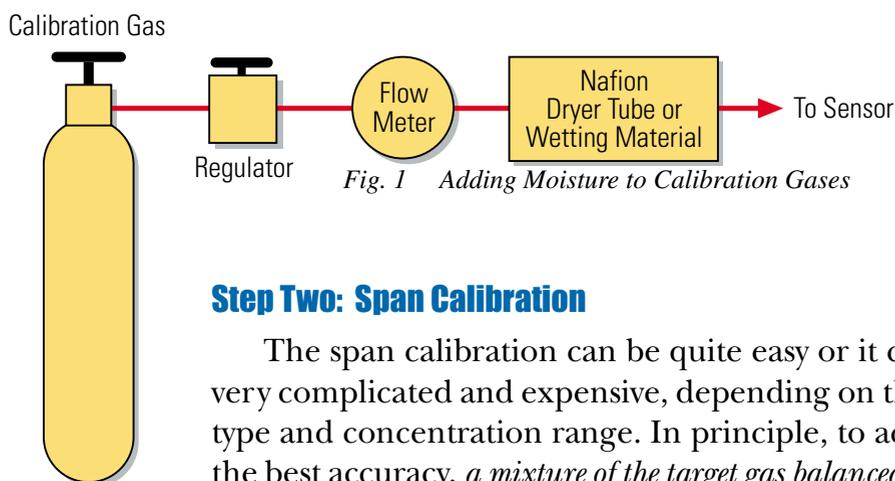
Fig. 1 Adding Moisture to Calibration Gases
