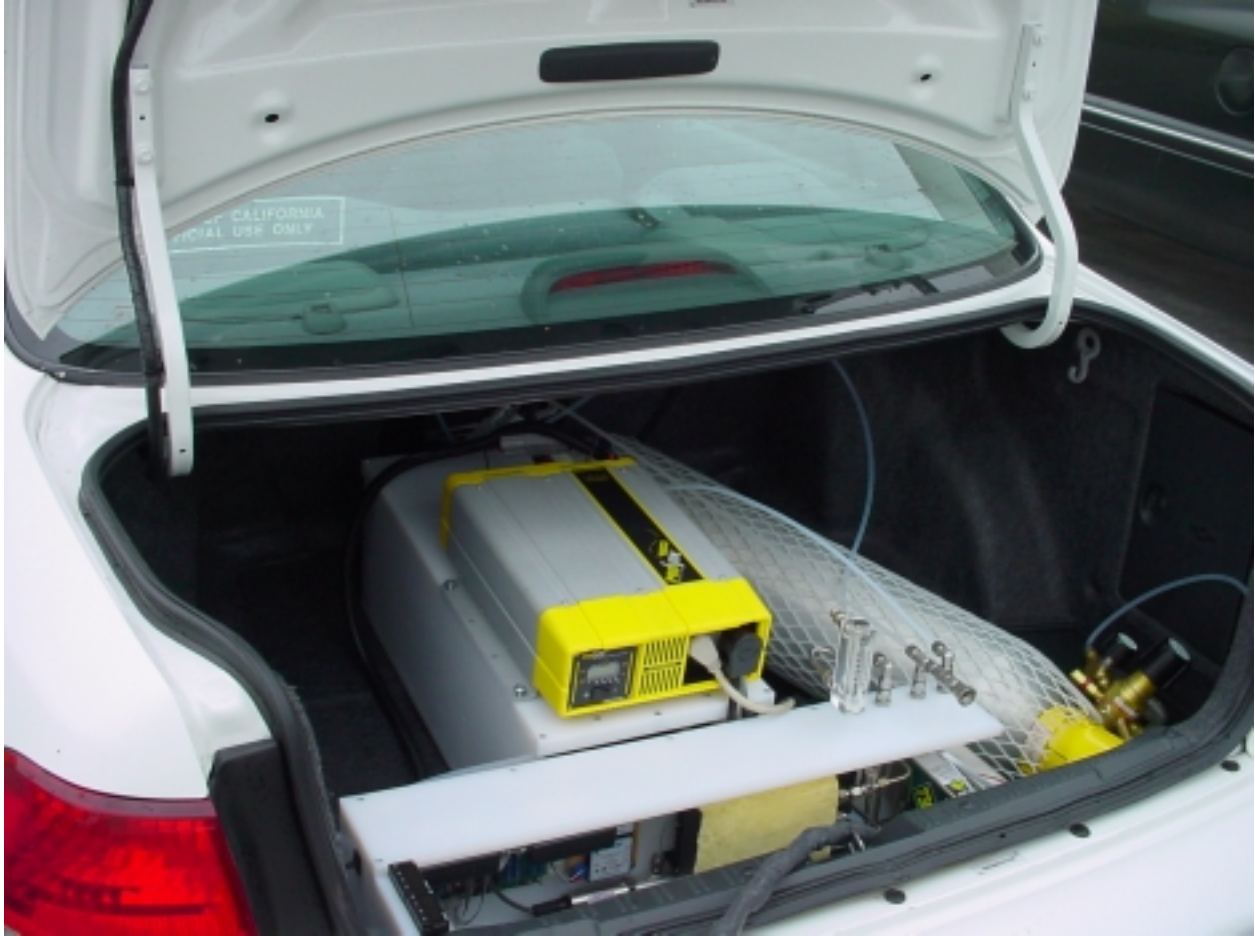
Figure 2-4. Conditioning system installed in cargo area of UCR test vehicle.
