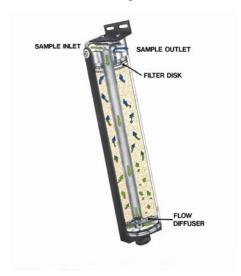
Phosphoric acid is very hydroscopic so it will draw water from the gas stream, creating some liquid phosphoric acid solution in the bottom of the scrubber. To avoid excess liquid formation, the scrubber should be heated, either by installation in a heated enclosure or by using a heated scrubber.
