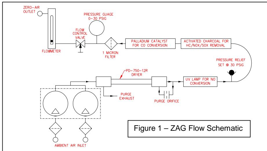
Maintenance requirements are minimal and easy to perform. There are two desiccant canisters, one of which needs to be replenished periodically; under normal use, it will last up to six months. The other desiccant canister contains a catalyst that is not consumable. The only other regular maintenance is to replace the particulate filter periodically. All other components in the system are designed to provide years of trouble-free service.
