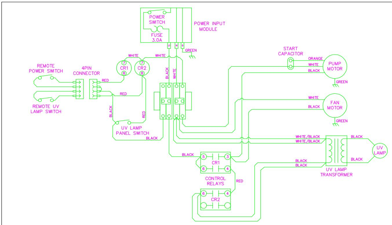
Figure 5 – ZAG Wiring Schematic
