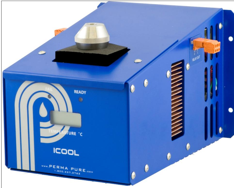
Accurate analysis of combustion samples and process control streams requires a method to remove the moisture from the sample without removing the gas components of interest. The **new** Integrator Series Thermo-Electric Cooler is an ideal way to decrease the moisture content of sample gases to a repeatable, stable dew point of 4°C (39°F).
