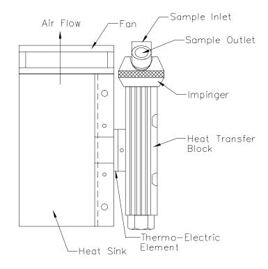
Figure 2: Heat Exchanger, Impinger and Heat Sink Assembly
