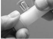
3. Gently pull the Nafion® tube element out of the housing just far enough to be able to remove the rubber ferrule. Remove the rubber ferrule.
