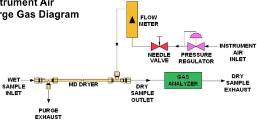
**Instrument Air** – Dried compressed or “Instrument” Air is typically found at most industrial plants and in many labs and serves as an excellent purge gas. The dew point of this purge gas is typically -40° to -45°C. Most of our performance curves have been made from test data using instrument air. We recommend the purge gas flow be 2-3x of the sample gas flow for optimal drying performance.
