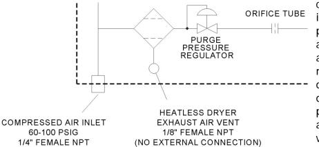
compressed air dryer. It is located in the lower part of the enclosure and provides dry purge air to the Nafion<sup>®</sup> membrane sample gas dryer. The heatless dryer operates on the pressure swing adsorption principle where one cylinder acts to dry the air under
