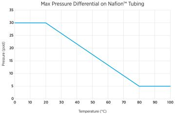
psid (psi-differential) = [sample gas pressure (psig) at inlet] - [sample gas pressure at outlet (psig)]
