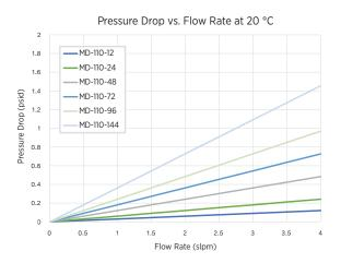
The performance curves above are based upon a sample inlet dew point of 20°C and purge flow rate of 2x the sample flow rate. Consult our team for operation with sample gases condensing above ambient temperature. psid (psi-differential) = [sample gas pressure at inlet (psig)] - [sample gas pressure at outlet (psig)], based on atmospheric pressure at outlet.
