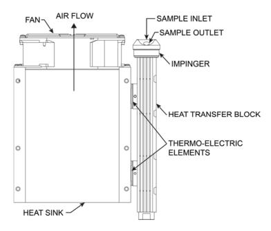
Figure A2: Impinger Diagram
