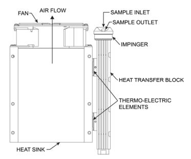
Figure 2: Heat Exchanger, Impinger and Heat Sink
