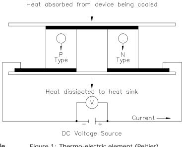
Figure 1: Thermo-electric element (Peltier)
