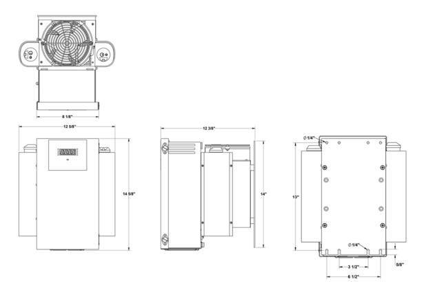
Figure A1: Model 8210D Dimensional Drawing
